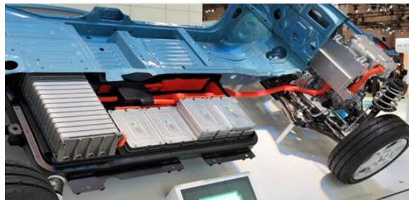
Figure 5 A lithium-ion battery pack incorporated into an electric vehicle
