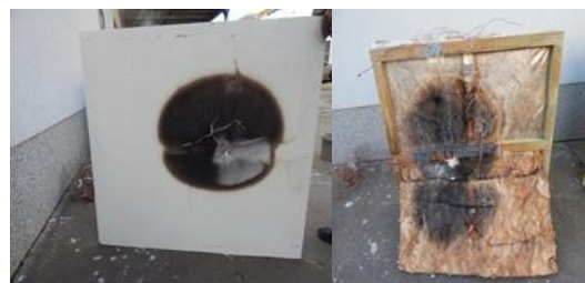
Fig. 12 Sample no. 2 – alternative 1 after testing (on right degradation of Entkopplung insulation board)
