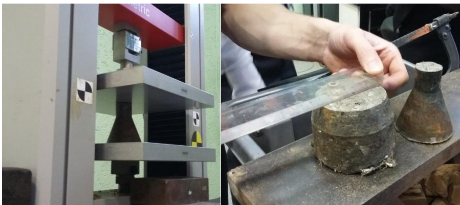
Figure 6 Uniaxial compressive strength test of the clog
