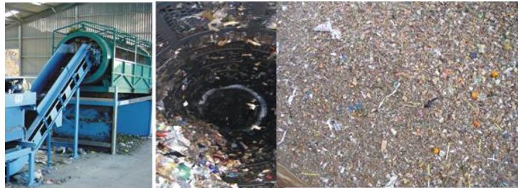
Figure 2 Separation of large (over 350mm) and small (smaller than 65mm) fractions at the screen
