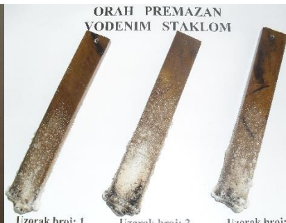
Fig 5 Samples with fire resistant coating after examination
