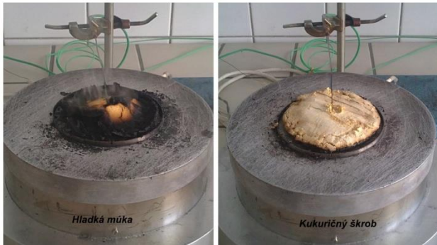
Fig. 3 Dust sample in sedimented form at 410 °C
