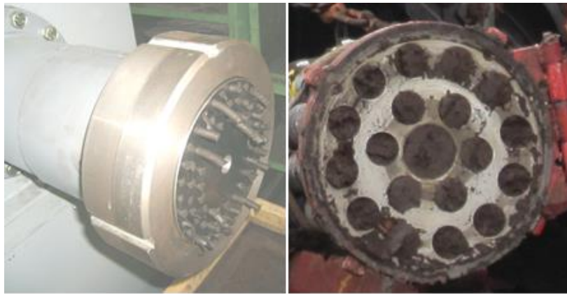
Figure 1 Clogged matrices reduce palletising to 50% matrix holes
