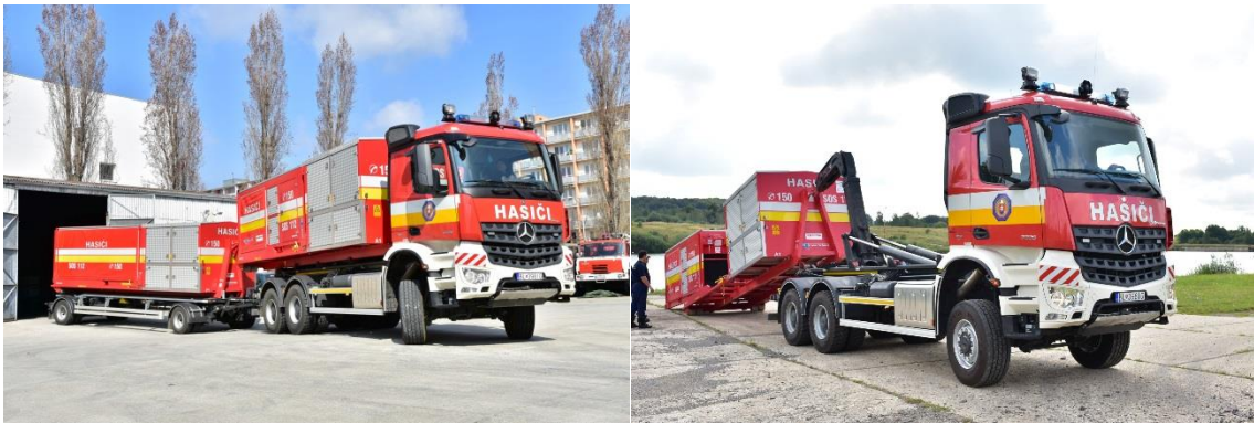
Fig. 2 System Hytrans a loading of container HydroSub 150 (author)
