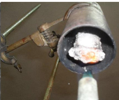
Fig 4 The swollen layer of water glass
