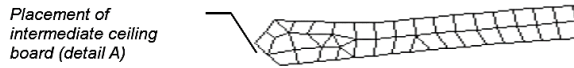
Fig. 8 Cross section and selection of nodes of the intermediate ceiling board of tunnel at modelling FEM
