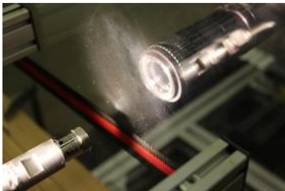
Fig. 3 Study of CNG release by high speed camera
