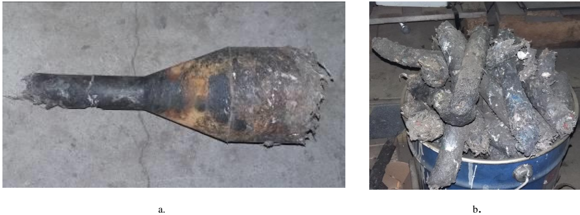
Figure 5 Stopper clog (a – stopper clog removed from the machine when the frame was cleaned, b – pellets produced on the machine)
