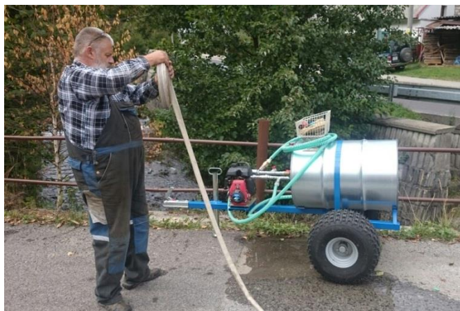
Fig. 3 Themselves made trailer for the quad vehicle POLARIS (photo DHZ Valaská)
