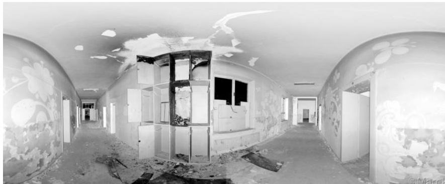
Figure 3 Infrared 3D scan - spherical view - 2nd fire scene [1]
