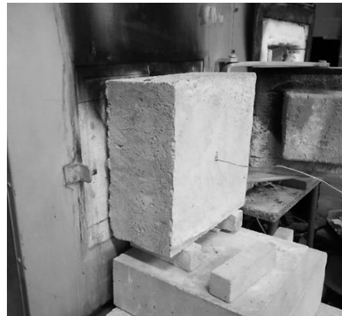
Figure 6 Arrangement of heating for the specimen
