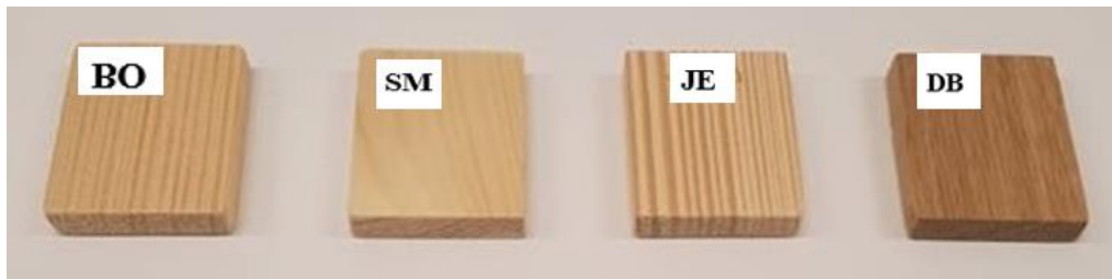
Fig 1. Photodocumentation of samples for the radiant heat source test (BO – pine, SM – spruce, JE – fir, DB – oak)
