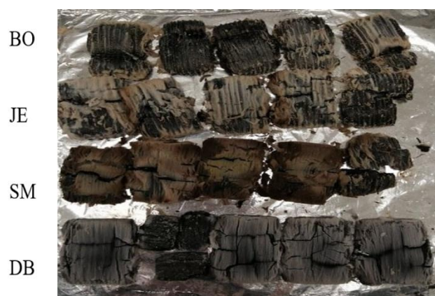
Fig. 3 Photo documentation of samples after the test by radiant heat source
