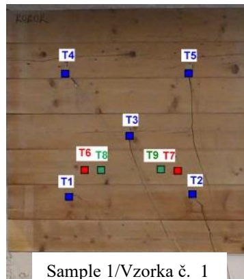
Fig. 2 Picture of the real sample with the positions of thermocouples
