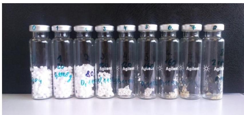
Fig. 1 EPS 100F samples after loading at particular temperature. (left to right: original sample, 20, 80, 100, 120, 140, 160, 180, 200 ^\circ\text{C} )
