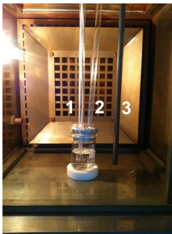
Fig. 2 Sample storage in a SEDEX safety calorimeter. 1 - Pt100 thermocouple, 2. glass rod for alcohol application, 3. thermocouple for sensing ambient temperature
