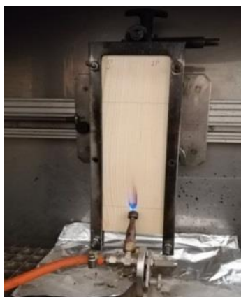
Figure 2 Demonstration of the impact of the test flame on the front face of the test specimens according to STN EN ISO11925-2
