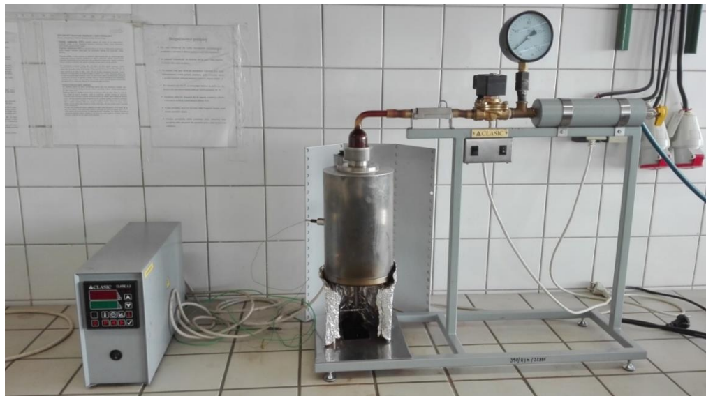
Figure 1 Device for determining the minimum ignition temperature of dispersed dust
