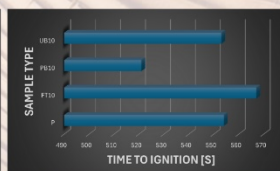
Fig. 3 Time to ignition of particleboard in dependence on the type of plastic filler
