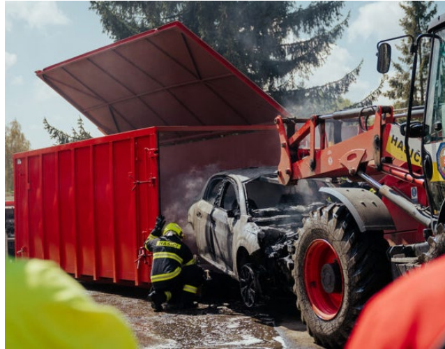
Obrázok 8 Kontajner na utopenie elektromobilu [18] Picture 8 Container for drowning of an electric car [18]
