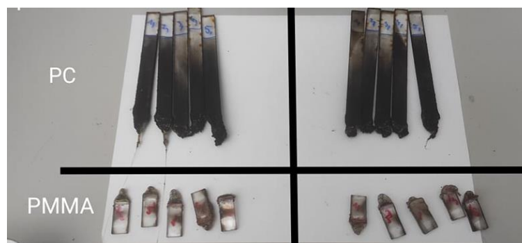
Fig. 4 PC and PMMA samples after testing with method B
