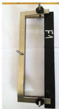
Obr. 9 Clamped specimen holder [9]
