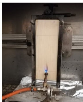
Fig. 2 Demonstration of the impact of a test flame on the front face of test specimens according to STN EN ISO11925-2
