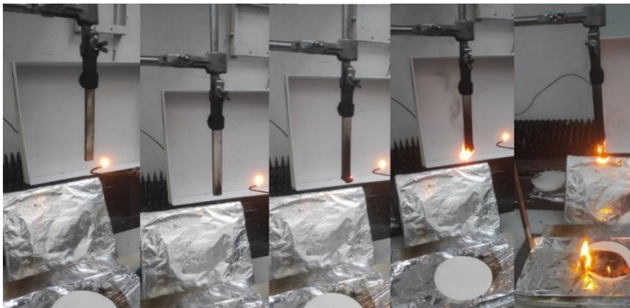
Fig. 8 PC burning pattern by method "B"
