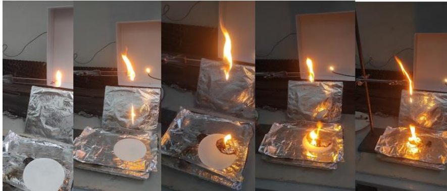
Fig. 1 PMMA burning pattern by Method "A"
