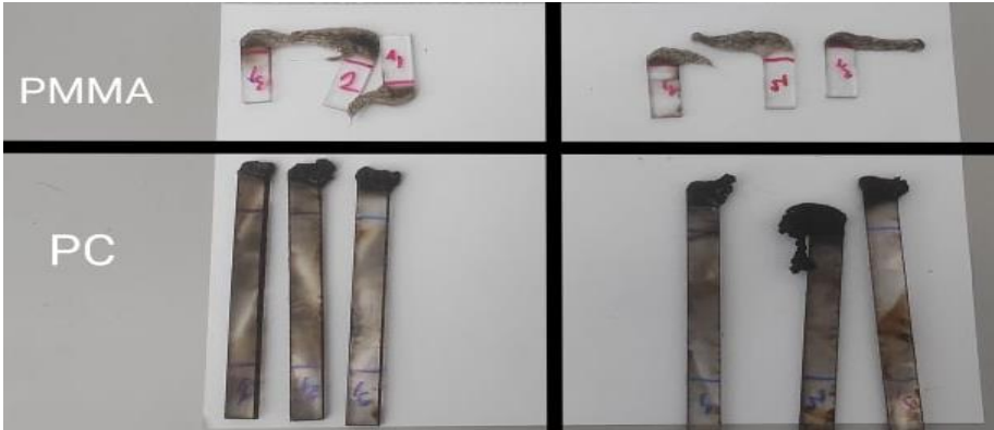
Fig. 6 PMMA and PC samples after testing with method "A"
