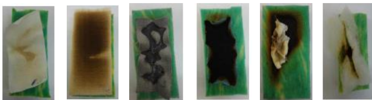
Fig. 5 Thermal degradation of samples (V1 –V6 left to right) + PUR NW – 15 cm
