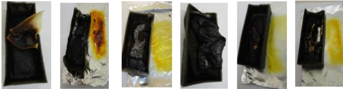
Fig. 8 Thermal degradation of samples (V1 –V6) + PUR S – 10 cm
