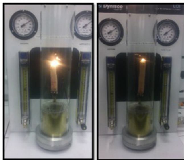
Obr. 1 Testovanie Deflammo KF 4545 pri LOI 25% obj, 26% obj.
