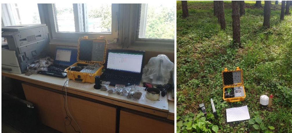
Fig. 1 Calibration process in the laboratory (left), field measurements of litter moisture content in the Arboretum Borova Hora (right)
