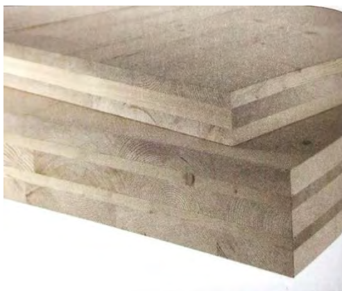
Obr. 11 CLT panel (Pavlas 2016)
