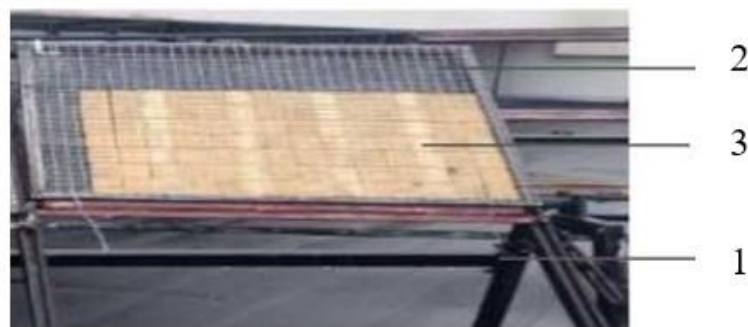
Fig 1. Storage of test samples: (1) adjustable metal stand; (2) metal frame with mesh for placing test samples; (3) test samples (untreated and treated with HR-Prof).
