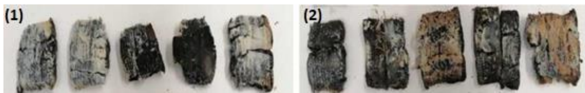
Fig 7. Spruce wood samples after the test (stored in an unprotected exterior): (1) untreated spruce samples; (2) spruce samples with HR-Prof application.
