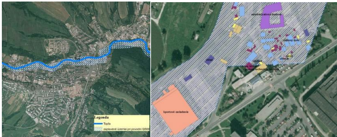
Figure 10.3 Result of flood zone calculation in the HEC-RAS model (Source: Majlingová, Galla, 2015)
