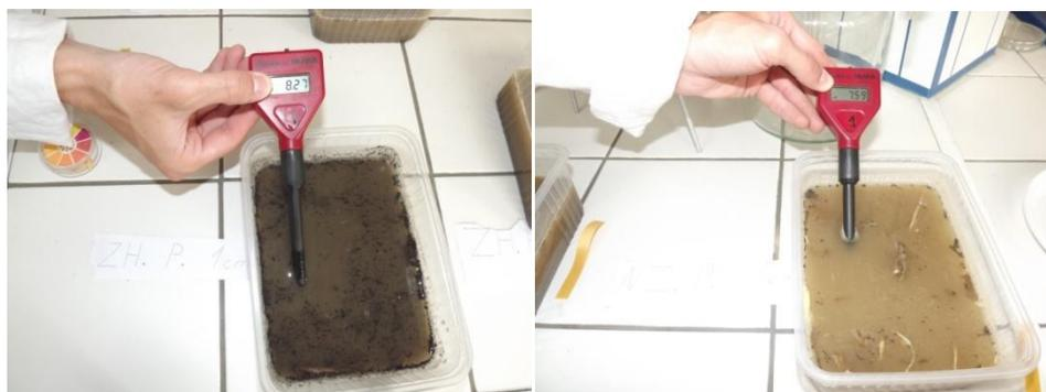
**Figure 4 Measurement of pH leachate with a pH meter (Source: Author, 2012)**
