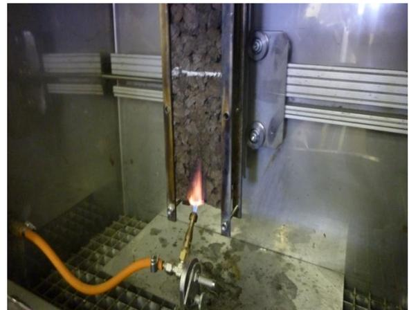
Figure 5 Testing technique of samples „on edge”
