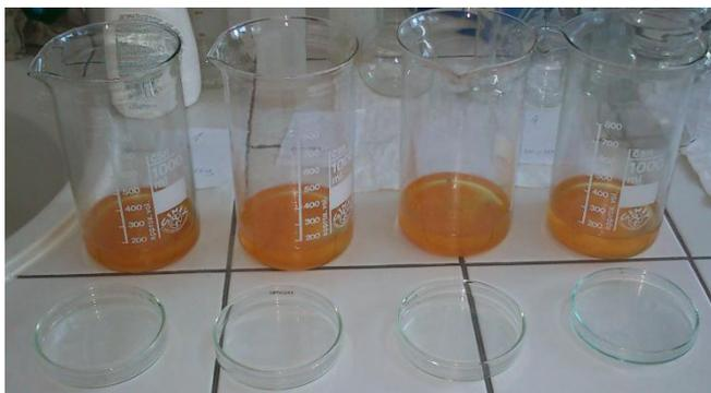
**Figure 5 A sample of fuel and sorbent UNI-SAFE after 10 minutes**
