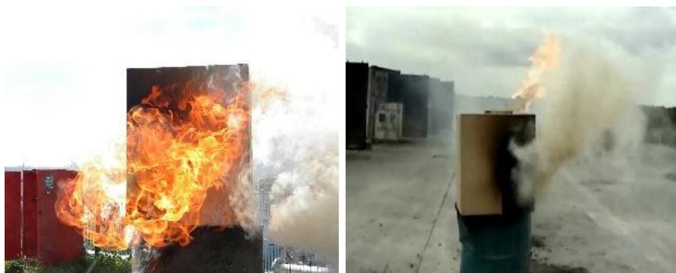
**Figure 7 Backdraft in mini-simulator**
