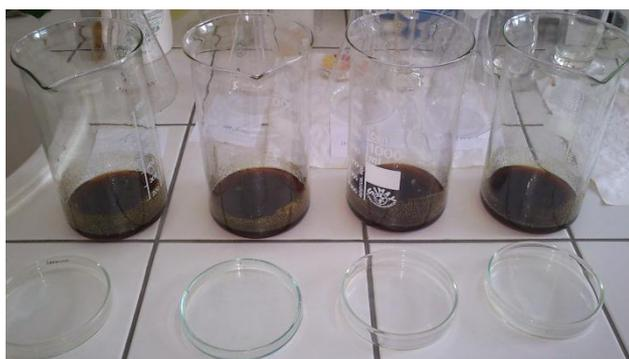
Figure 7 fuel and sorbent samples UNI-SAFE after 10 minutes
