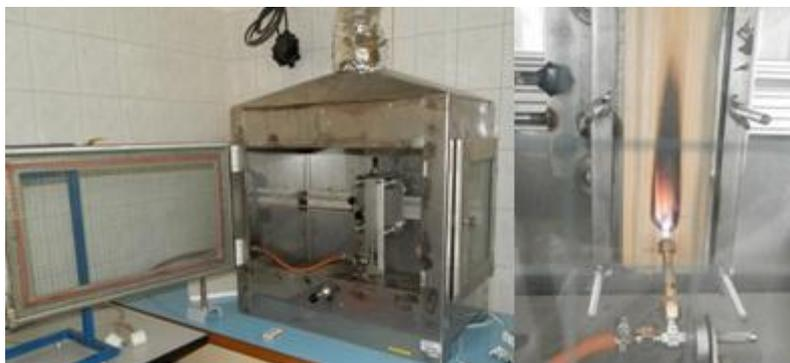
Figure 5 Device for testing the reaction of combustible products for fire
