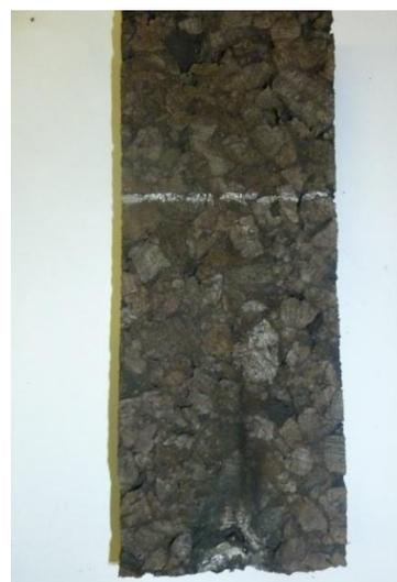
Figure 7 The place of flame contact after 5 minutes of testing „on edge“
