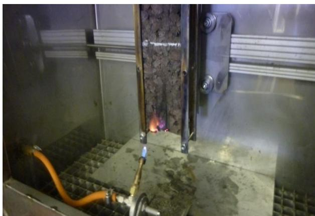
Figure 6 Sample was in flames even after the source of heat was withdrawn
