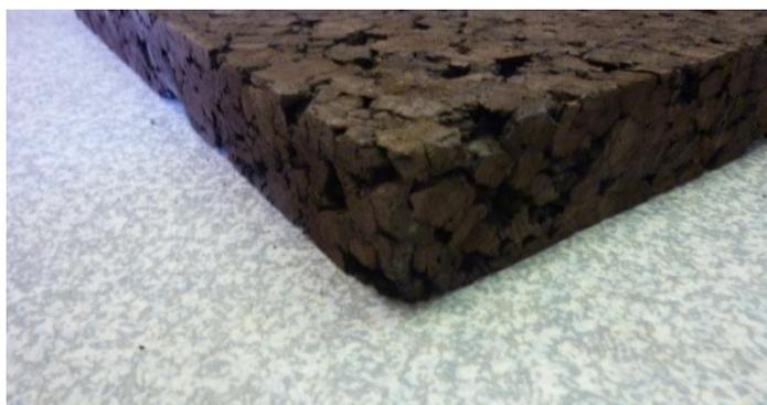
**Figure 1 Sample no. 1 – insulation corkboard**
