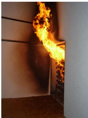
**Figure 2 Pictures of tests for the detection method in the testing laboratory (eg, the flame tip to the second floor above the fire floor)**
