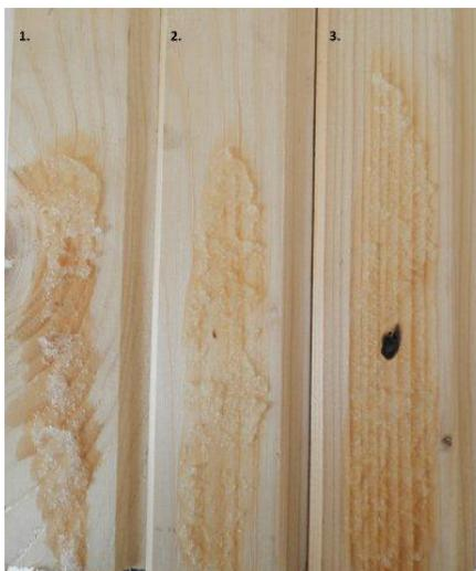
**Figure 9** The samples of wooden boards with fire extinguishing gel Hydrex after attempting
