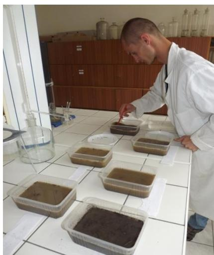
**Figure 3 Preparation of extracts from soil samples (Source: Author, 2012)**
