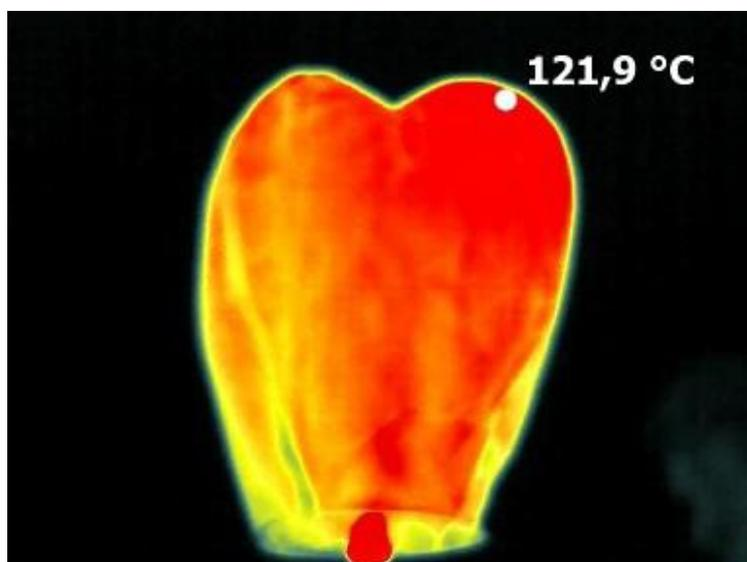
Figure 6 The peak temperature of the casing sky lantern
