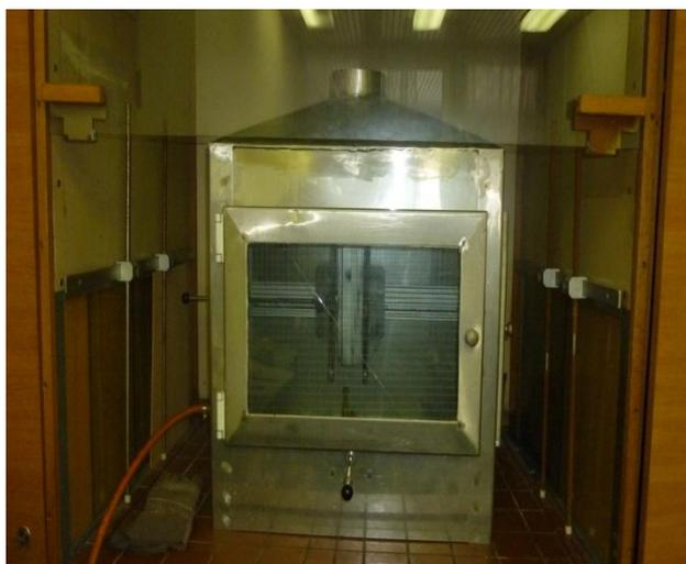
**Figure 3 Testing devices according to STN EN 11925-2**
