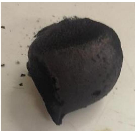
**Obr. 21** Sample after isothermal heating at 250 °C
