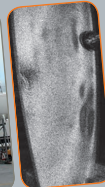
Resin-filled honeycombs in aluminum honeycomb panel
