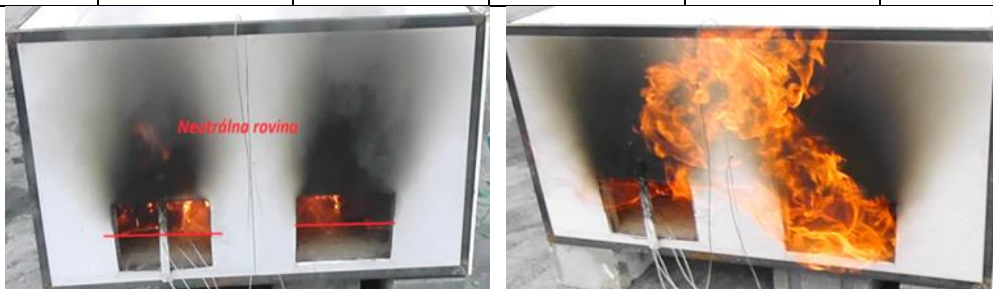
Figure 2 Neutral plane and the phenomenon of flashover
